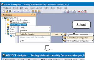
Right-click "Module Configuration" on the Workspace window, and select [Module Configuration] ⇒ [New] ⇒ [L Series Module Configuration] in the shortcut menu.
