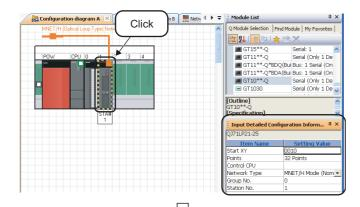
Click the network module (QJ71LP21-25) on "Configuration diagram A".
