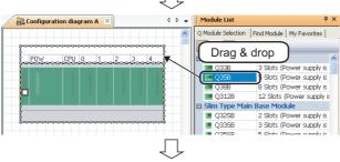
Select the base unit ( Q35B) from the Module List window, and drag and drop it onto the Module Configuration window.
