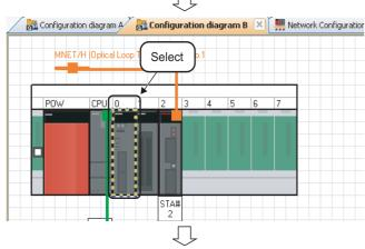
8. Select [Q Module Configuration] ⇒ [Parameter] ⇒ [Multiple CPU Parameter Setting] in the menu bar.
