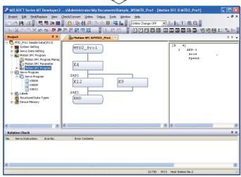
The motion controller project, which is allocated to CPU No. 2 on the Module Configuration window, is activated and the target motion SFC program is displayed.
