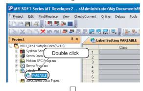
Double-click "VARIABLE" on the Navigation window of MT Developer2 to display the Label Setting window.
