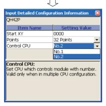
2. Set the parameters on the Input Detailed Configuration Information window.
