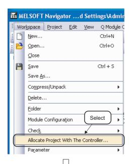
Select [Workspace] ⇒ [Allocate Project With The Controller] in the menu bar to display the "Allocate Project With The Controller" dialog box.
