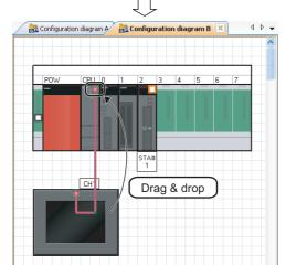
the Module List window, and drag and drop it onto the connection port of the GOT unit.
