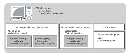
To use system labels in iQ Platform supporting engineering environment MELSOFT iQ Works, utilize system labels registered in MELSOFT Navigator from projects (Top-down design method), or register global labels defined in projects as system labels (Bottom-up design method).
