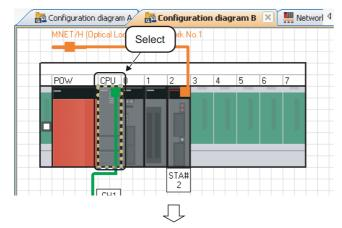
1. Select the CPU No. 1 controller on the Module Configuration window.
