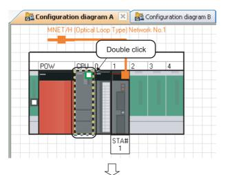
On the Module Configuration window, double-click the controller to which a programmable controller project is allocated.
