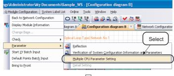
2. Select [Q Module Configuration]  $\Rightarrow$ [Parameter] ⇒ [Multiple CPU Parameter Setting] in the menu bar.
