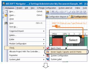
Select[Workspace]⇒[Check]⇒[Power Supply Capacity and I/O Points] in the menu bar.
