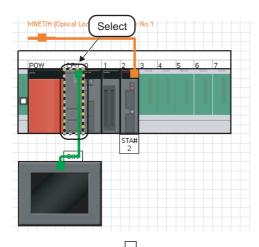
On the Module Configuration window, double-click the controller to which a programmable controller project is allocated.
