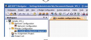
3. Enter "L module configuration diagram A" to change the module configuration diagram name.
