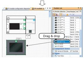
4. Select modules from the Module List window, and drag and drop them onto the Module Configuration window following the same procedure in the step 4 through step11 in section 3.4.2.
