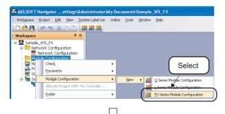
Right-click "Module Configuration" on the Workspace window, and select [Module Configuration] ⇒ [New] ⇒ [FX Series Module Configuration] in the shortcut menu.
