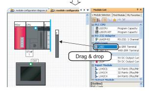
4. Select modules from the Module List window, and drag and drop them onto the Module Configuration window following the same procedure in the step 4 through step11 in section 3.4.2.
