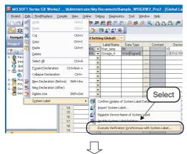
Select [Edit] ⇒ [System Label] ⇒ **[Execute Verification Synchronous with** System Label] in the menu bar of GX Works2.
