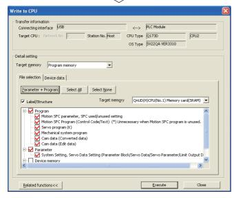
On the System Configuration window, right-click the controller to which a motion controller project is allocated, and select [Online] ⇒ [Read]/[Write]/ [Verify] in the shortcut menu.
