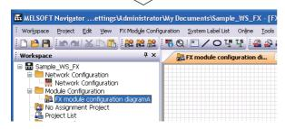
3. Enter "FX module configuration diagramA" to change the module configuration diagram name.
