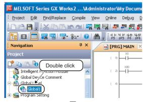
2. Double-click "Global1" on the Navigation window of GX Works2 to display the Global Label Setting window.
