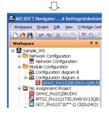
Right-click the controller on the Module Configuration window, and select [Allocate Project With The Controller] in the shortcut menu to display the "Allocate Project With The Controller" dialog box.
