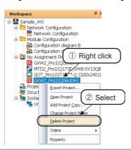
Right-click the project name on the Workspace window, and select [Delete Project] in the shortcut menu to delete the project. Allocate projects in the workspace to controllers on the Module Configuration windows.
