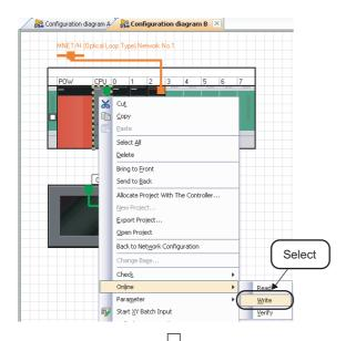
On the System Configuration window, right-click the controller to which a programmable controller project is allocated, and select [Online] ⇒ [Read]/[Write]/[Verify] in the shortcut menu.
